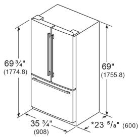
\* Add 1-15/16" (49mm) in the back measurements for proper ventilation
