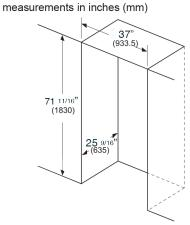
Leave 2" (50.8) gap at the top and 1  $\frac{3}{6}$ " (34.9) behind the refrigerator for proper ventilation.
